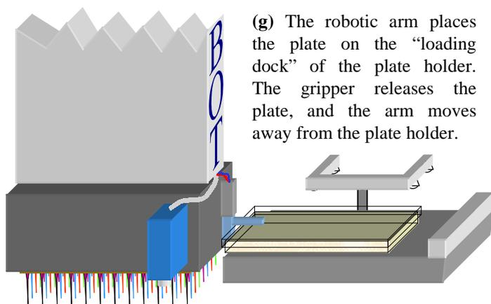
(g) The robotic arm places the plate on the “loading dock” of the plate holder. The gripper releases the plate, and the arm moves away from the plate holder.
