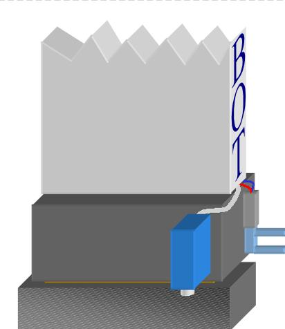
(e) Upon completing the wash/sterilization cycle, the arm places the picking head into the blow drier. The warm air released by the blow drier causes evaporation of residual ethanol left on the pins.
