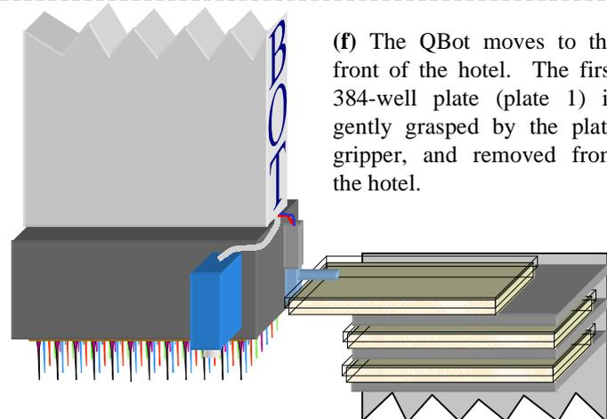
(f) The QBot moves to the front of the hotel. The first 384-well plate (plate 1) is gently grasped by the plate gripper, and removed from the hotel.
