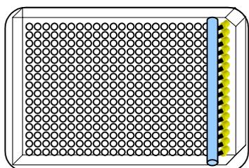
The mechanical stage moves the plate underneath the manifold. The manifold itself does not move during operation.
