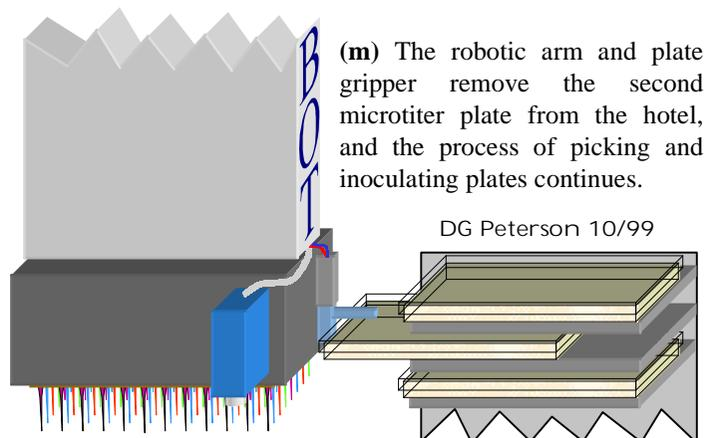
(m) The robotic arm and plate gripper remove the second microtiter plate from the hotel, and the process of picking and inoculating plates continues.
