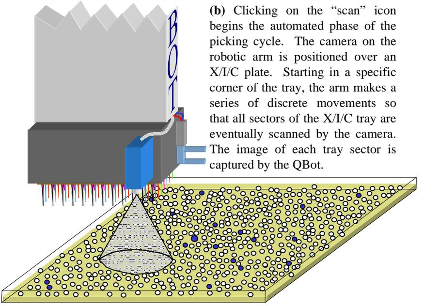
(b) Clicking on the “scan” icon begins the automated phase of the picking cycle. The camera on the robotic arm is positioned over an X/I/C plate. Starting in a specific corner of the tray, the arm makes a series of discrete movements so that all sectors of the X/I/C tray are eventually scanned by the camera. The image of each tray sector is captured by the QBot.
