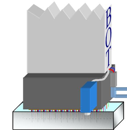
(d) Once the picking cycle is initiated, the QBot’s first order of business is to sterilize the picking pins. In brief, the robotic arm places the bottom of the picking head (*i.e.*, the pins) into the ethanol wash bath. The arm makes a series of short, jerky movements effectively moving the pins back and forth through the bath. Groups of clustered bristles lining the bottom of the bath enhance the cleaning process.
