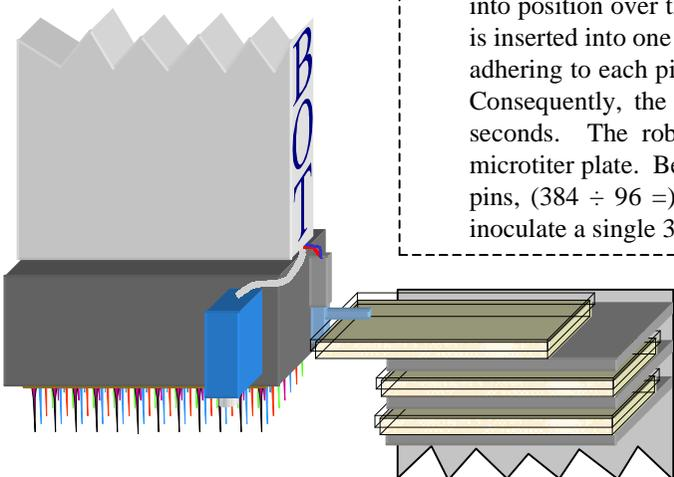
(l) Once the first plate has been completely inoculated, the lid manipulator puts the lid back on the plate. The plate holder shifts the plate back into “transport position” and the plate is picked up by the plate gripper on the robotic arm. The inoculated plate is placed back into the same slot of the hotel from which it was originally removed.
