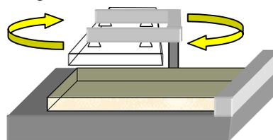
(i) The lid manipulator places the lid on a “low profile” resting pad adjacent to the plate holder. The manipulator remains attached to the lid.
